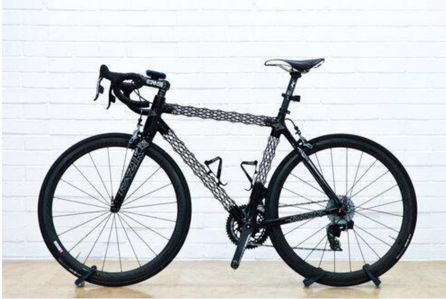
Figure 3. Photograph of an IsoTruss bicycle frame. The IsoTruss geometry reduces bicycle frame weight by 51% compared to a traditional aluminum frame.
